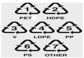
NOTE: PET-Polyethylene terephthalate, HDPE-High density polyethylene, V-Vinyl (PVC), LDPE- Low density polyethylene, PP-Polypropylene, PS-Polystyrene and Other means all other resins and multi-materials like ABS (Acrylonitrile butadiene styrene), PPO (Polyphenylene oxide), PC (Polycarbonate), PBT (Polybutylene terephalate) etc.
